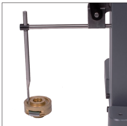
Depth measurements with accessories 930.2108 and 930.2105
