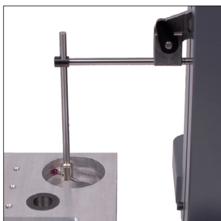
Internal groove measurements with accessories 930.2108, 930.2110 and 905.2207
